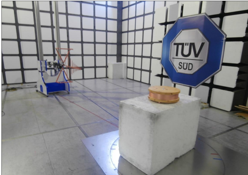
Figure 8 - Test Setup - 30 MHz to 1 GHz
